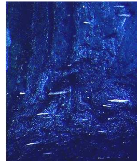
Blue brittleness test for non-metallic inclusions
