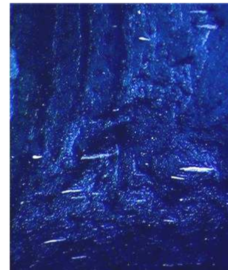
Blue brittleness test for non-metallic inclusions
